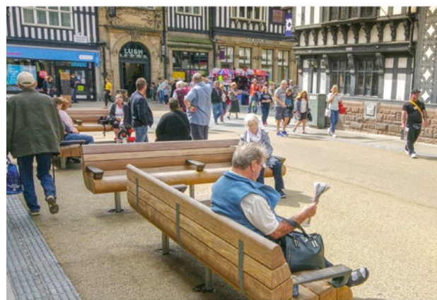
Tactile edge to delineate pedestrian and vehicle movement zone
