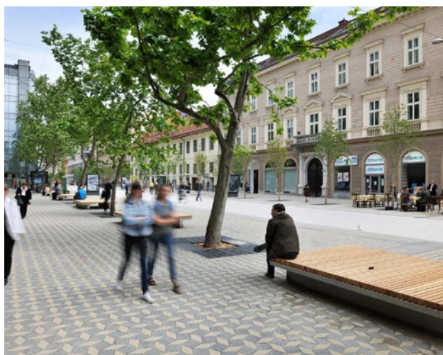
Patterned paving along the footpaths provides clear distinction between the clear central movement corridor.
