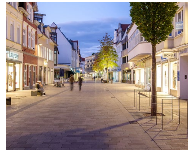
'Slow and fast' routes demarcated by subtle changes in paving unit sizes and contrasting edges.
