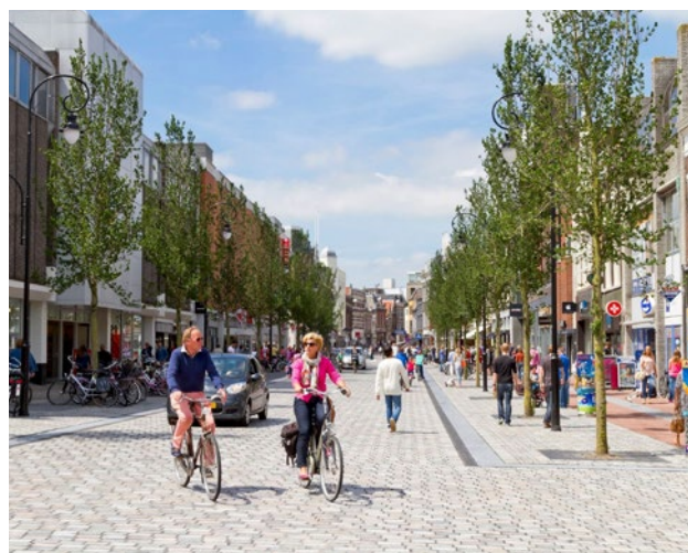
Tactile edges located along the shared movement corridor provide visual distinction between pedestrians, cyclists and vehicles.
