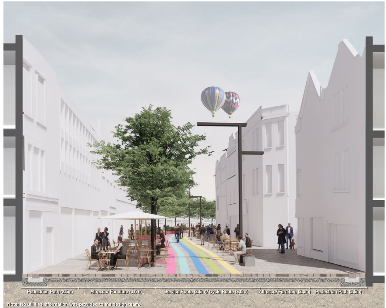
Cross sectional perspective of the street showing alfresco dining, flexible modules and fixed seating.
